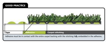
Application - Apply sufficient adhesive to the back of the carpet to totally cover and fill the backing ridges.
