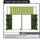
Seam joints - Ensure that the carpet joins down the centre of the tape and that sufficient adhesive is covering the tape - ideally a minimum of 24cm width of adhesive onto a 30cm Seaming Tape.
